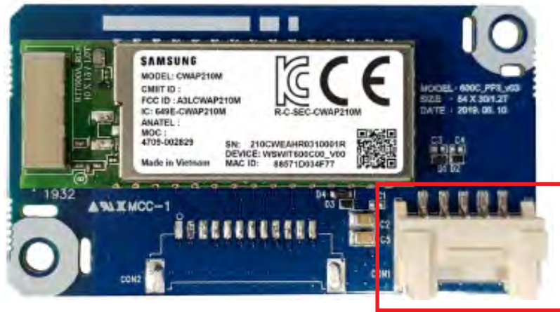
CON1 : MAIN PBA ↔ Wi-Fi Module #1 TX / #2 RX / #3 RST / #4 GND / #5 12V
